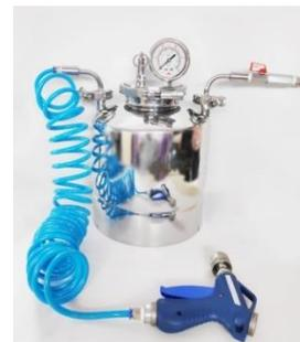
Dispensing Pressure Vessel holds liquid for filtration through pressure operated filter holders made of 316 SS, In-built NRV, Pressure Relief Valve Silicon O-ring and base is mounded with Styrene butadiene rubber. Used to spray concentrated jet of ultra clean solvent or rinse solution on surfaces for cleaning. A-one filter holder
